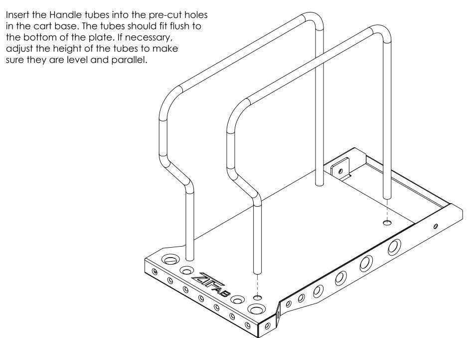
**Step 5A: Tacking Tubes** Ensure that tubes are 90\* to the base and parallel to each other. Then tack weld into position. -Parallel 90° 1000
