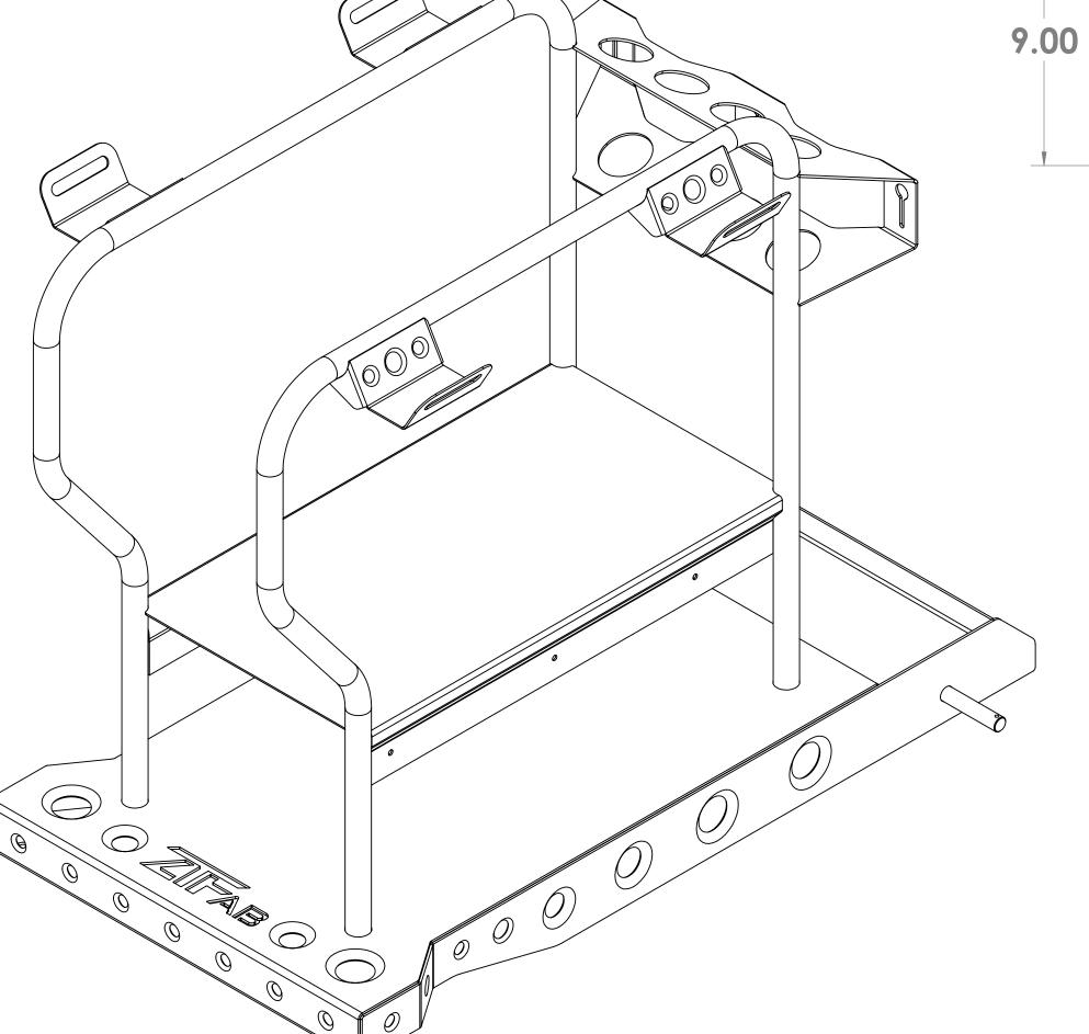
Use clamps or spacers to keep the shelf in position. Tack weld the shelf to the tubes.
